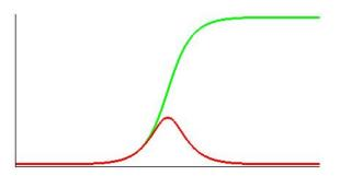
The lower curve represents  $u_x$  (and is similar in general shape to the energy density) and the upper curve represents the soliton itself smoothly interpolating u = 0 to  $u = 2\pi$ .
